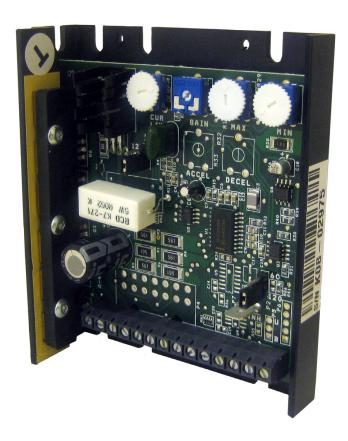
DB Series is a family of brushless DC motor control s designed to provide commutated power and variable speed control for standard 3 phase brushless DC motors. The controls operate in a basic open loop or closed loop configuration with either 60° or 120° brushless DC motors. Compact, economical, and efficient, the DB Series is ideal where high torque, high speed and quiet operation are needed.
