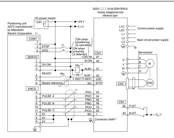
\*1: The ALM signal is output for five seconds or less when the power is turned ON. Take this into consideration when designing the power ON sequence. The ALM signal actuates the alarm detection relay "1Ry" to stop the main circuit power supply to the SERVOPACK.
