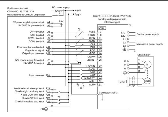
\*1: The ALM signal is output for five seconds or less when the power is turned ON. Take this into consideration when designing the power ON sequence. The ALM signal actuates the alarm detection relay "1Ry" to stop the main circuit power supply to the SERVOPACK.
