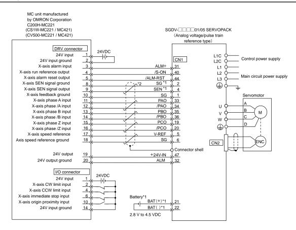
\*1: Use a battery when using an absolute encoder.
